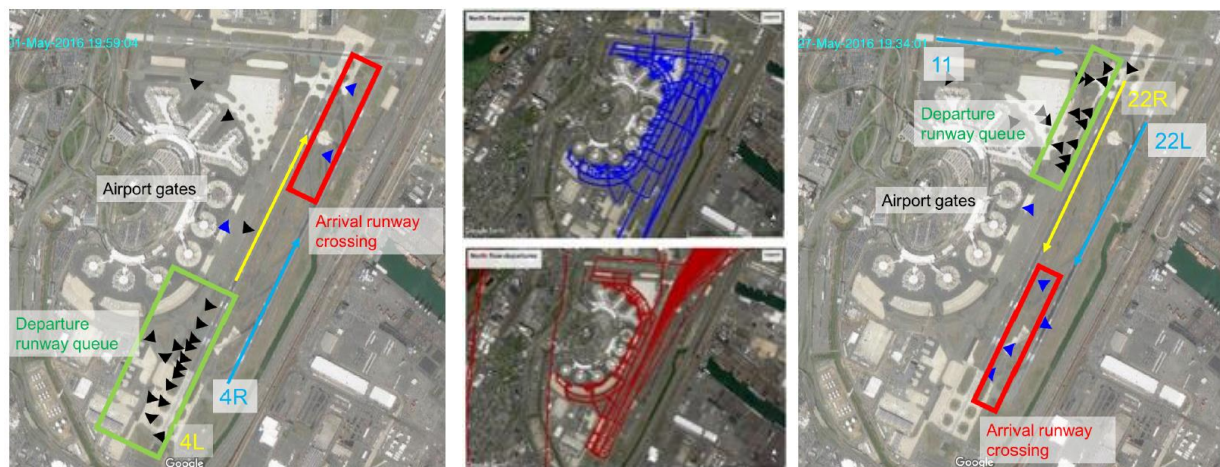
Figure 107. (Left) Airport layout for EWR in North-Flow; (Center) Taxi-in and taxi-out trajectories in the North-Flow, and (Right) Airport layout in the South-Flow.
